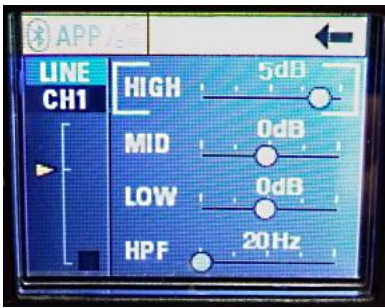
Fig. 6 CH1 High band EQ, +5 dB
