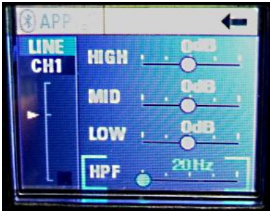
Fig. 14 HPF Filter Band
