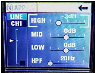
Fig. 7 CH1 High band EQ, -3 dB
